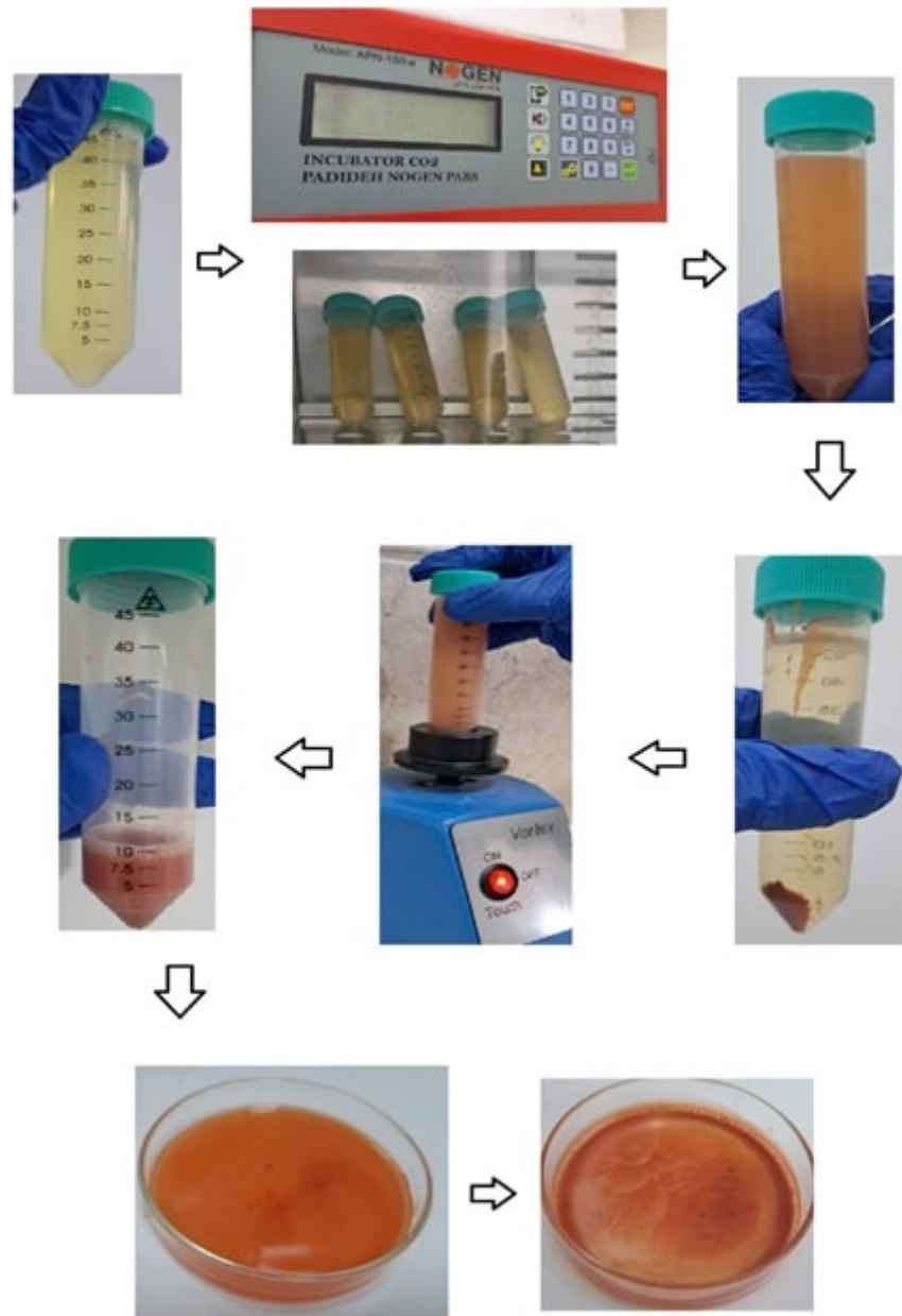
Figure 1. Incubation, centrifugation, washing, and drying of SeNPs synthesized by the green method
